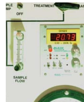
State-of-the-art monitoring technology, such as the Analox 10000 oxygen monitor ensures our patients are kept safe during operations.
